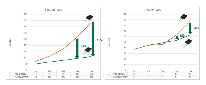
Figure 6. Switching Loss Comparison ( $E_{ON} \& E_{OFF}$ ): TO-247-3L vs TO-247-4L Kelvin Source Package under V<sub>DD</sub>=1200V, V<sub>GS</sub>=-3V/+18V, R<sub>G</sub>=2 $\Omega$ , FWD : PCH120S10D1(1200V/10A SiC Diode) and I<sub>D</sub>=5~25A
