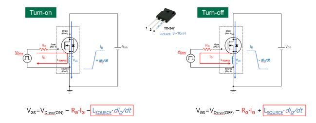
Figure 2. Source Inductance influence of TO-247-3L Package at Switching Turn-On & Turn-Off Transient
