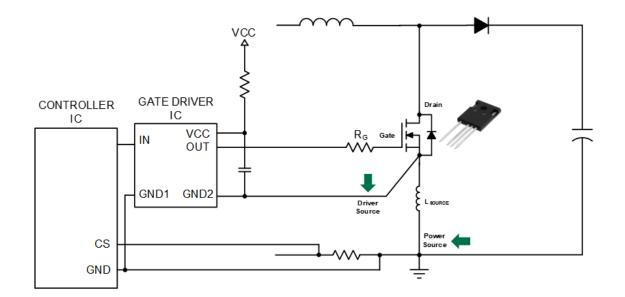
Figure 9. Drive circuit of Boost PFC for TO-247-4L Kelvin Source Package
