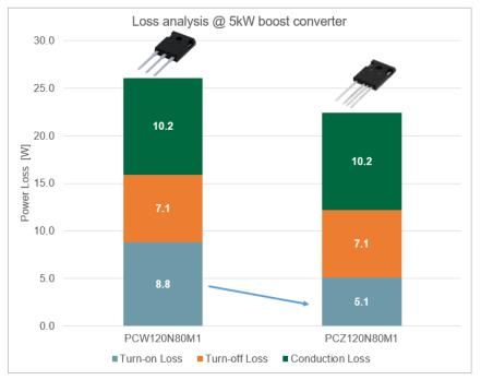
**Figure 8.** Power Loss Analysis under Full Load in Boost Converter of 5kW Solar Inverter
