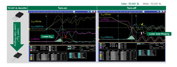
Figure 7.Switching Waveforms Comparison at Turn-On (left) and Turn-Off (right) transient<br/>: TO-247-3L vs TO-247-4L Kelvin Source Package under  $V_{DD}$ =1200V,  $V_{GS}$ =-3V/+18V,  $R_G$ =2 $\Omega$ ,<br/>FWD : PCH120S10D1(1200V/10A SiC Diode) and  $I_D$ =5~25A
