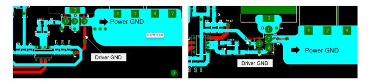
Figure 4. PCB Layout of Gate Driving Circuit : TO-247-3L (left) vs. TO-247-4L (right)
