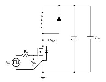
**Figure 5.** Double Pulse Switching Test Board
