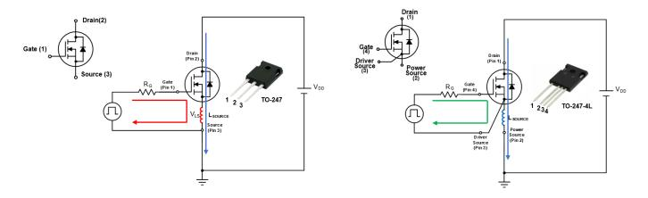
Figure 3. Gate Driving Circuit : TO-247-3L (left) vs. TO-247-4L (right)
